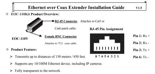
> Easy to install, no IP and MAC address configuration required
